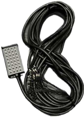
Figure 4: A 32-channel (24 inputs, 8 outputs) multicore cable. The box would be placed on the stage, the 'tails' are plugged into the mixing desk.
